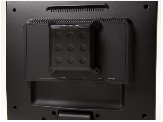
The above picture shows the terminal attached to the monitor mount. This is done by sliding the terminal on the attachment clips and pushing it down to secure it.
