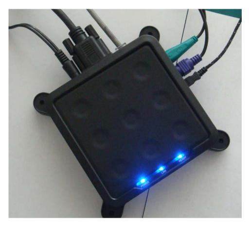
The access terminal must be connected via Ethernet to the host PC. This can be done using an Ethernet switch, a router, or some other network connection method.
