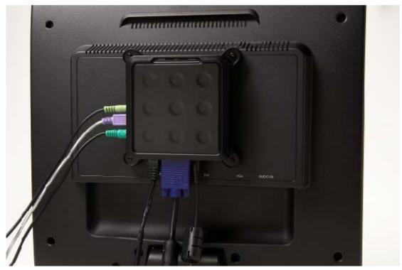
The above picture shows the JF-ETP-5100B on the mounting bracket, secured with the mounting collar, and all cablesconnected.
