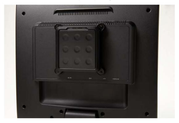
The above picture shows the mounting collar holding the terminal in place with the four black screws.
