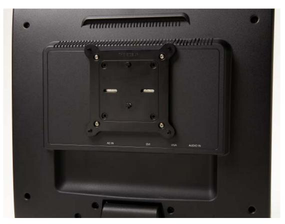
The above picture shows the monitor mount attached to the back of the monitor with the four silver screws. Note that the black attachment clips are oriented vertically. Also, note there are holes in the monitor mount that support a 100 mm mount and a 75 mm mount.
